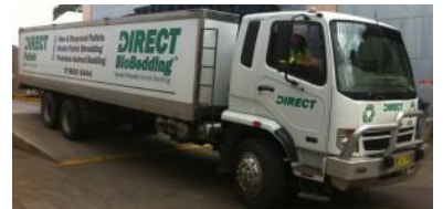
Our 40 m 3 , Low height (2.7m) Walking Floor – Our Small "Direct BioBedding" Delivery Truck
